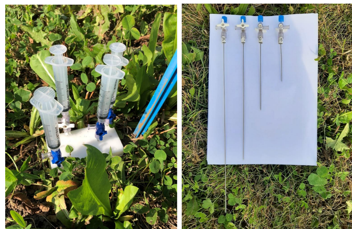
Figure 2. Detail of the needles used to collect N 2 O concentration in the soil profile.
